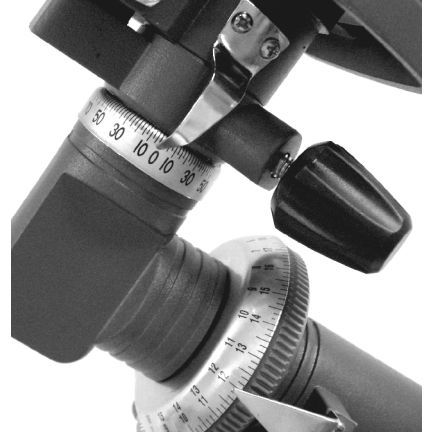
Figure 4-10 Dec. circle at top and R.A. circle at bottom
